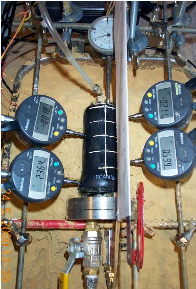
Figure 5. Picture of the infiltration test with swelling allowed.
