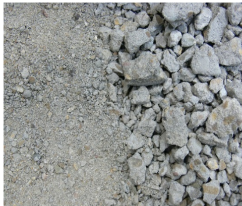
Fig. 1. Recycled concrete aggregate fractions 0/4 (left side) and 0/16 (right side).
