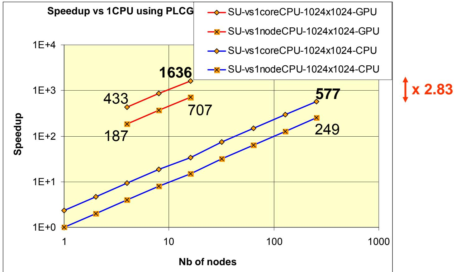
With 16 GPU nodes: speedup vs 1-core-CPU reaches 1636,
