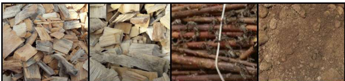
Figure 1. From left to right: pine chips, birch chips, willow stems, hydrolysis lignin.
