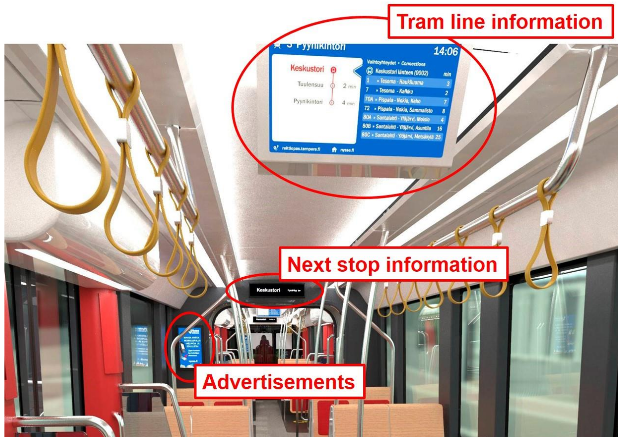
Figure 9. Displays and their purposes in the tram (Photo: Tampereen Raitiotie Oy).
