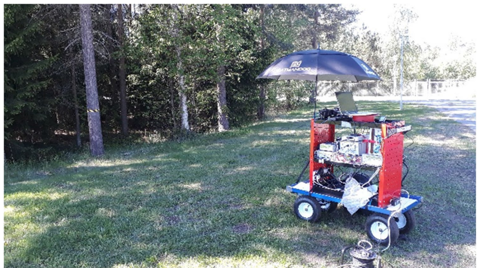
Fig. 4 The VTT SPAD LiDAR equipment on a carriage and targeted at the sample tree
