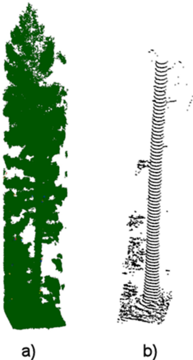
Fig. 5 The 3D points of the sample tree measured with ZEB Horizon (a) and VTT SPAD LiDAR (b)
