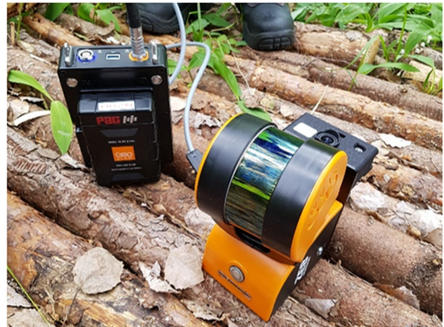
Fig. 1 ZEB Horizon hand-held scanner head and data acquisition unit
