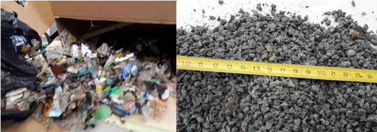
Figure 4. Reject from plastic recycling (F-SRF) going to feed zone of MODIX (left) and grains (right) after MODIX-treatment and crushing.
