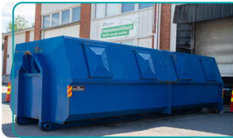
Figure 32 Covered skip used in LSJH's sorting stations
