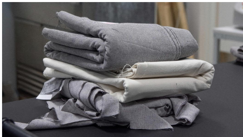
Figure 44 Fabric samples made out of mechanically recycled textiles and test ©Taru Marttila
