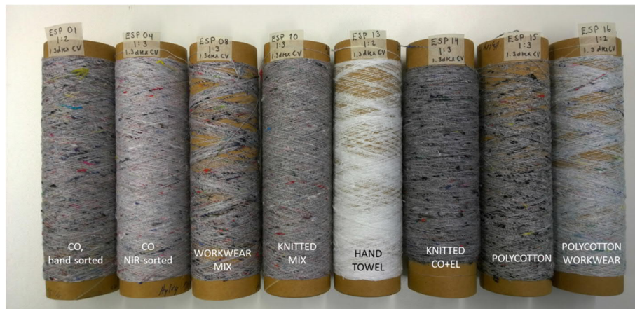
Figure 42 Ring spun yarns from mechanically opened fibres from post-consumer textiles. Mechanically opened fibres were blended with virgin viscose fibres (length 40 mm) in ratios of 1:3 and 1:2.
