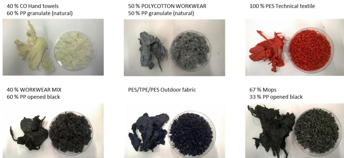
Figure 50 Examples of compacted (left) and grinded (right) materials
