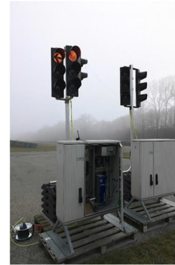
Figure 11. Traffic lights with C-V2X
