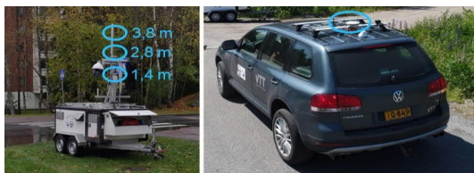
Figure 2. Antenna installations in the LTE-V2X trials. The trailer installations are shown on the left, and the 5G and LTE-V2X antennas of the test vehicle “Martti” were located on the roof.
