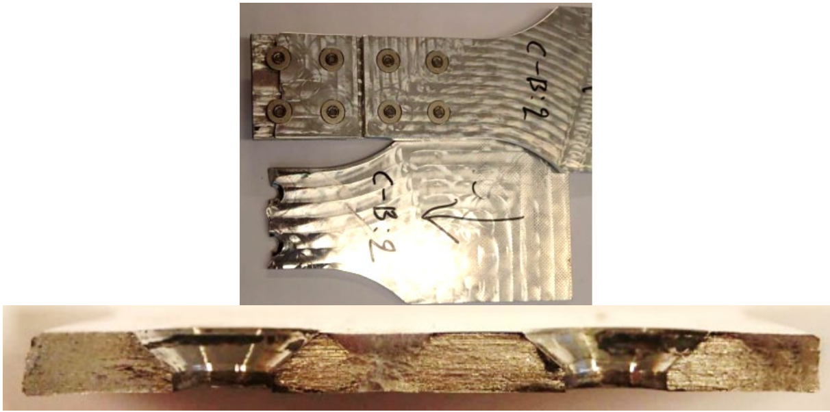
Figure 53: Failure mode I in C-B specimen. Figure courtesy of Saab Aeronautics.
