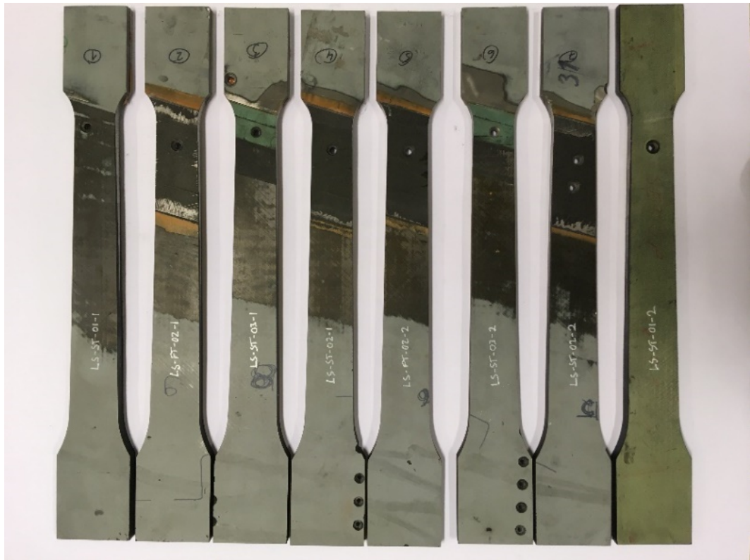
Figure 63: Finalized test specimens. Figure courtesy of Patria Aviation.
