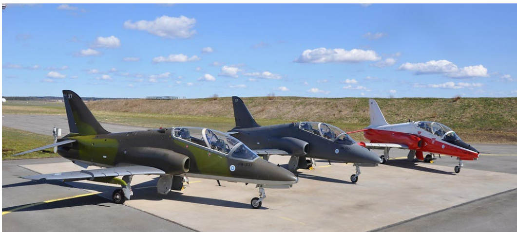
Figure 8: BAE Systems Hawk advanced jet trainer variants in the FINAF fleet (from left to right): Hawk Mk.51, Hawk Mk.51A, and Hawk Mk.66. Figure courtesy of the FINAF.
