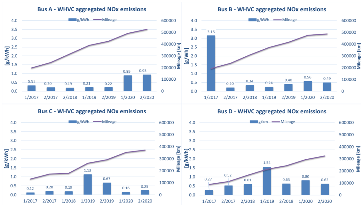
Figure 18: Aggregated (cold + hot cycle) NO x emissions on WHVC. Euro VI limit value on WHTC is 0.46 g/kWh.
