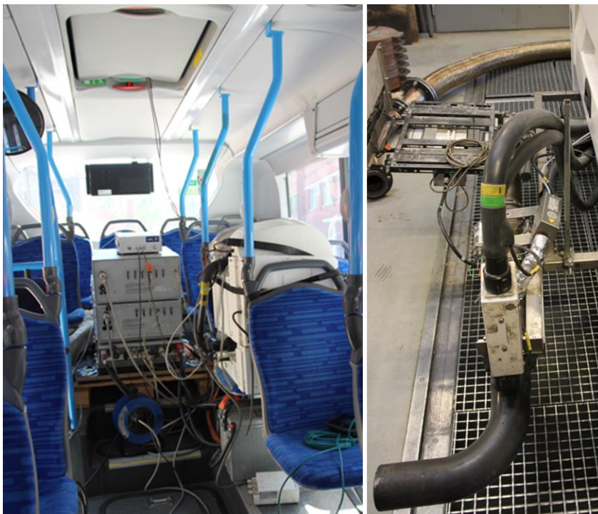
Figure 4: Exemplary installation of the PEMS device. Emissions analyzers inside the bus and EFM installed at the back of the bus.
