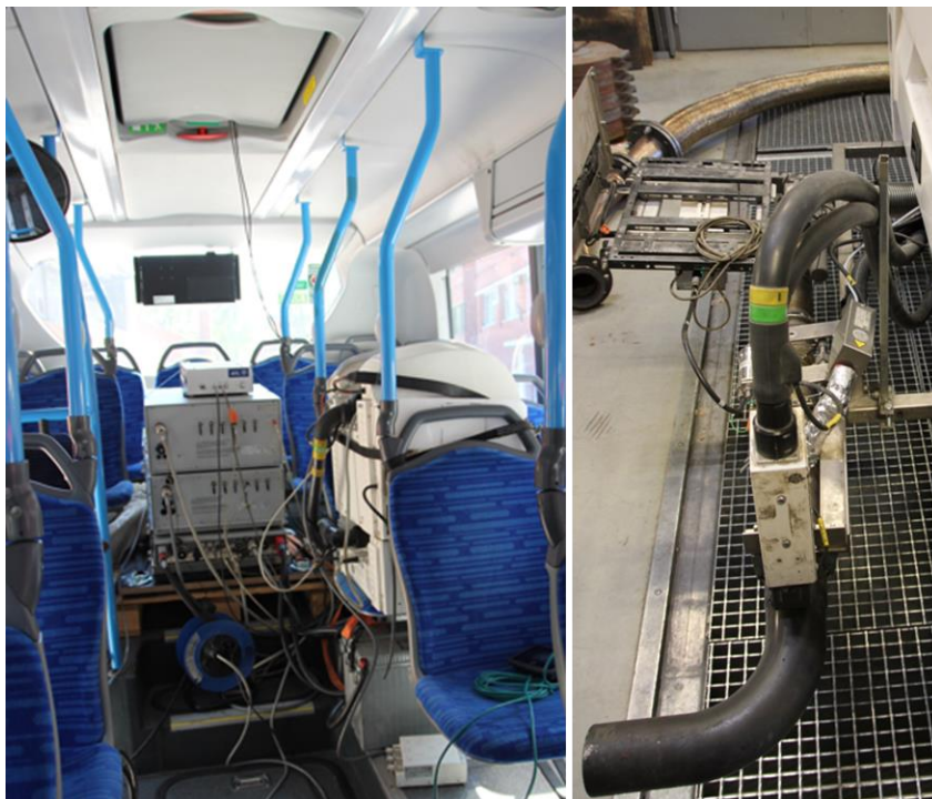
Figure 4: Exemplary installation of the PEMS device. Emissions analyzers inside the bus and EFM installed at the back of the bus. Speed profile and location on a map are shown in Figure 5 and Figure 6. Two of them describing typical operation in HSL traffic. Third route was fulfilling the requirements of the Euro VI ISC testing. First typical HSL traffic route was following one
