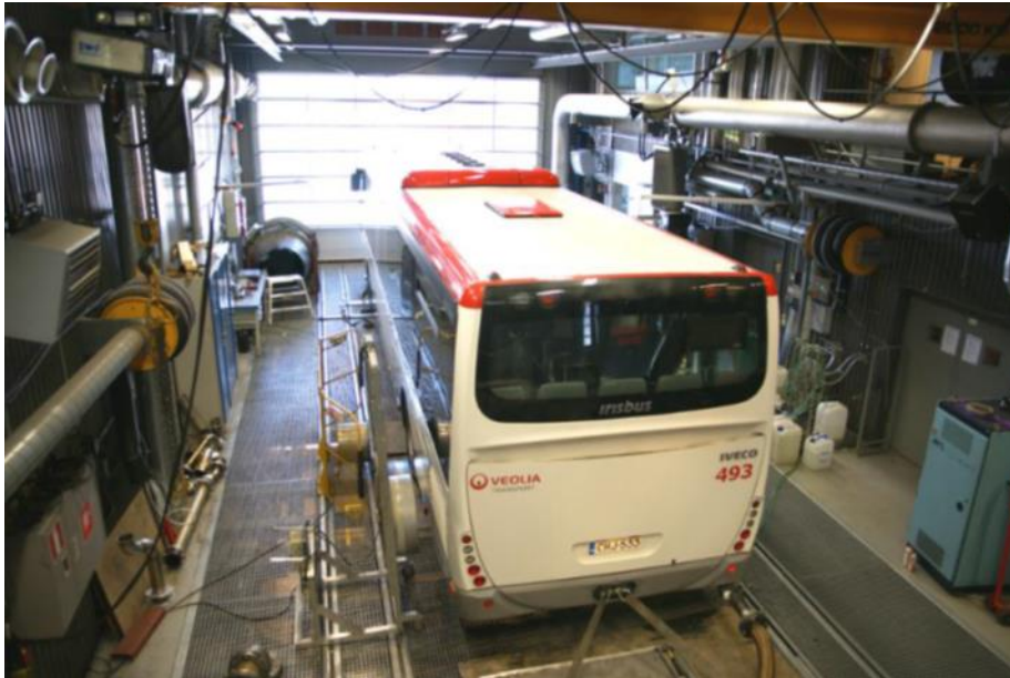
Figure 1: View of the HD chassis dynamometer. The CVS tunnel can be seen on the upper right corner of the figure.
