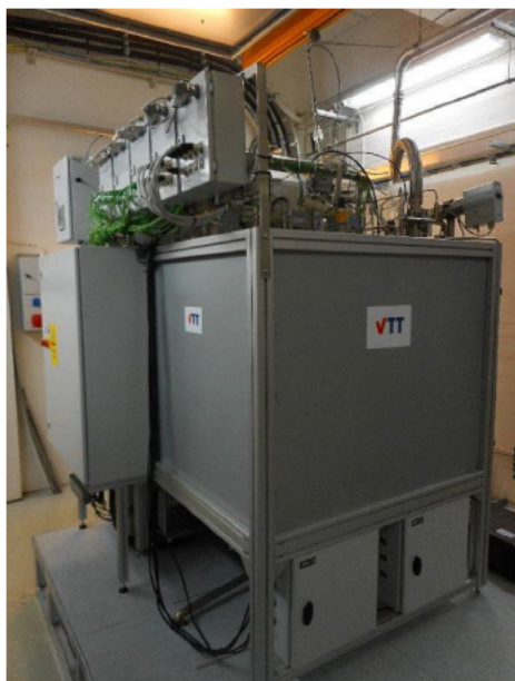
FIGURE 8 Movable “10-foot container” size rSOC system
