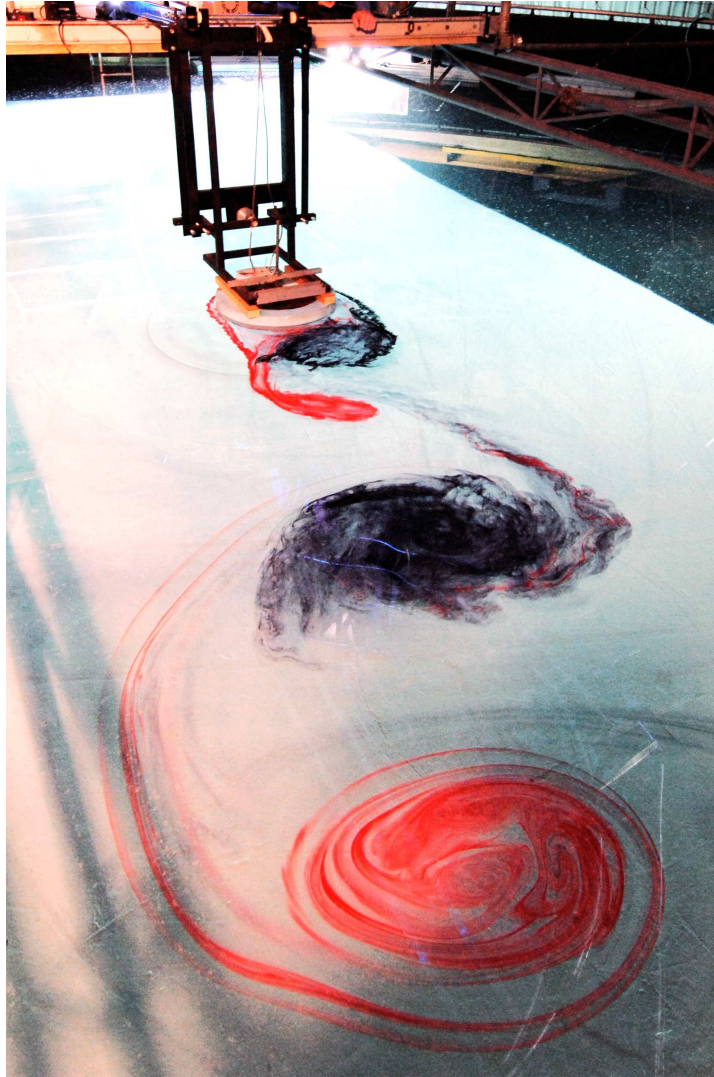
FIG. 6.5: A front view of a dye experiment for Ro \simeq 1 , Re \simeq 10000 , and Bu \simeq 6.5 .
