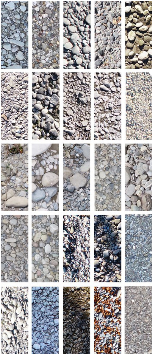
Figure 3. Example image tiles ( 1.25\text{ m} \times 0.5\text{ m} ) with 0.25\text{ cm} ground sampling distance. Each of the 25 example tiles is taken from a different gravel bar.
