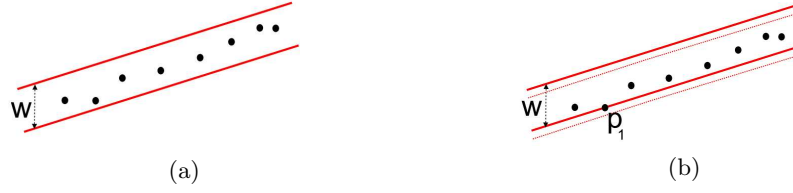
Fig. 2. A digital line that has no critical point (a), and its translated digital line that has one critical point p_1 (b).
