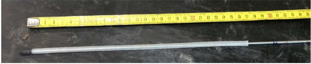
Figure 3.21. Needle for the placement of vertical drains.
