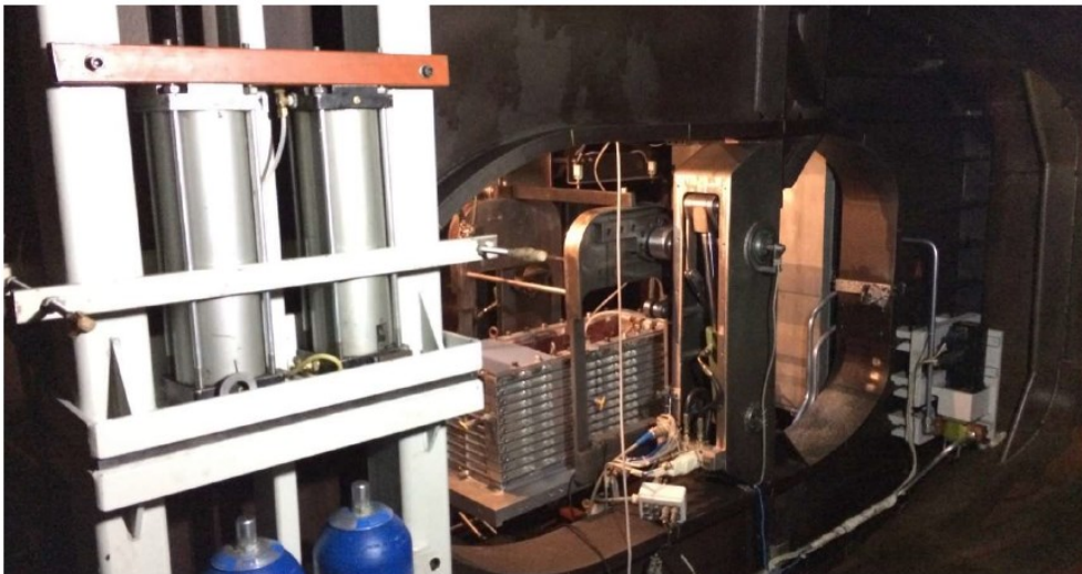
Figure 3.24. Induced partial saturation (IPS) system of ISMGEO (Airoldi et al., 2018b).
