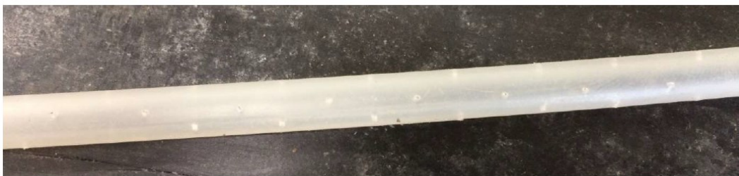
Figure 3.20. Silicon pipe for vertical and horizontal drains.
