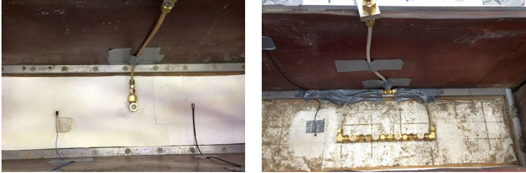
Figure 3.25. Nuzzles for induced partial saturation.
