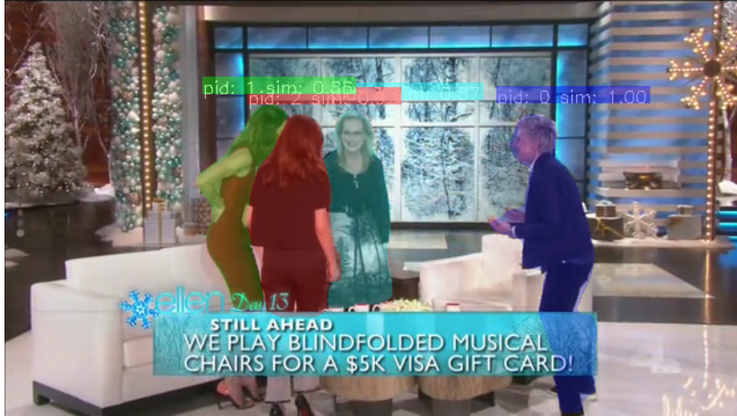
Figure 5.4. The output of the spatial segmentation model with a heavily occluded input.
