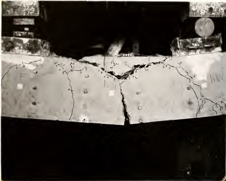
FIG. B23. VIEW OF BEAM B2 AFTER FAILURE
