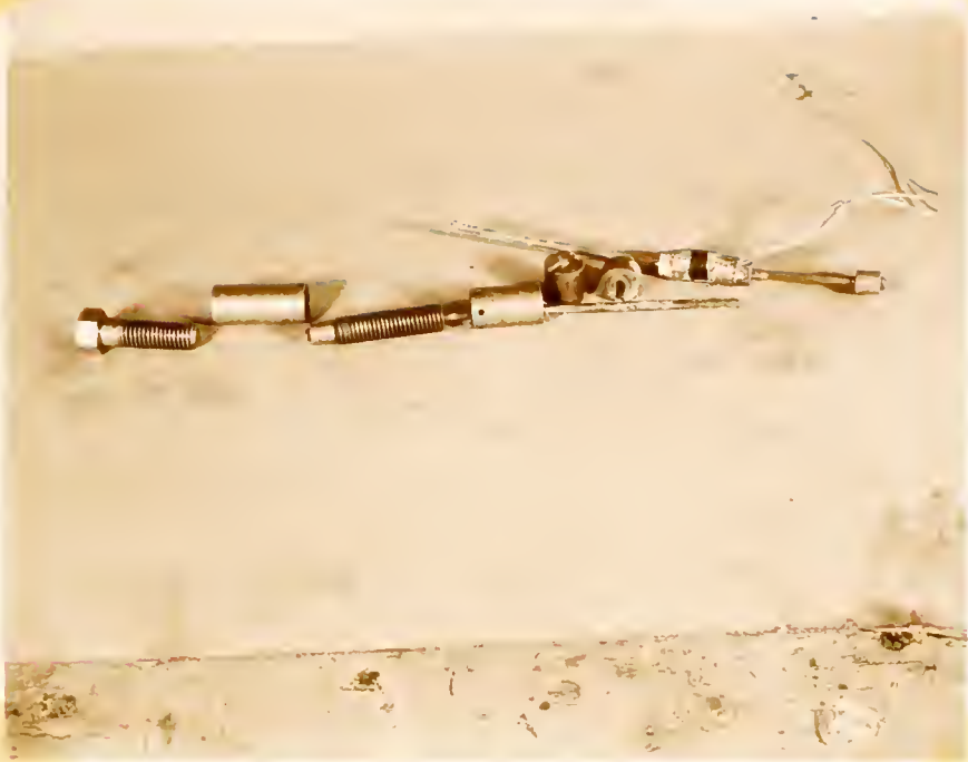
FIG. B10. VIEW OF SHIMMING DEVICE AND DYNAMOMETER
