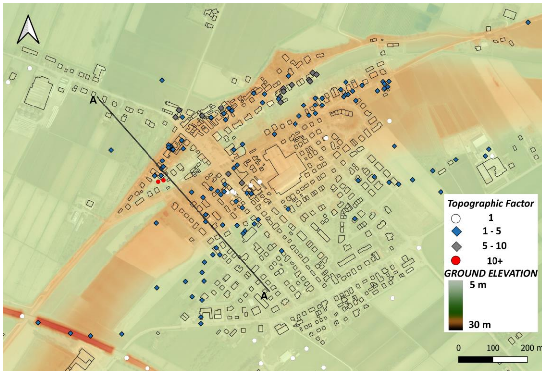
Figure 6-18 Evaluated Topographic Factors (TF) in the district of S. Carlo and trace of the section “AA” displayed in Figure 6-17.
