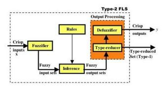
Figure 1. Scheme of type-2 fuzzy logic system (FLS). *Source:* Castro *et al.* (2008).
