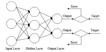
Figure 2. Schematic neural network of a kind of back propagation. *Source*: Erb (1993).
