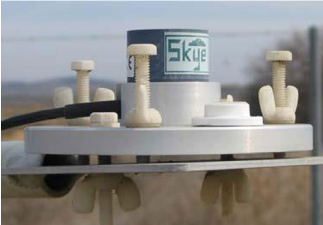
Figure 2. SKYE SP1100 or CM3 pyranometers. Source: REDAREX (Extremadura Regional Government).
