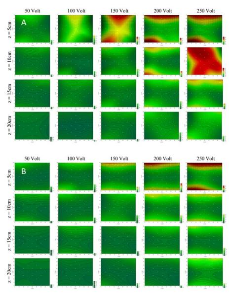
**Figure 6.** Pattern of the electrical signal intensity inside a portion of the palm tree after providing different electric voltage (*i.e.*, 50, 100, 150, 200 and 250 V) for direct current (A) and alternating one (B). The signals were registered by the electrodes inserted at different depth from the cutting plane.
