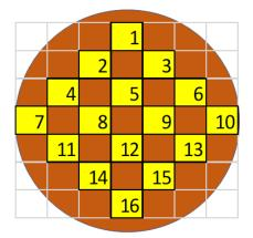
Figure 3. Areas of the stem portion tested for conductivity
