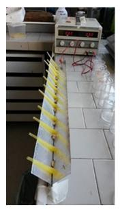
Figure 2. Larvae electrocution tests on aluminium plates and with plastic separators.
