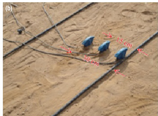
Figure 2. Installation of EasyAG probes in the plot: (a) buried drip line; (b) drip line on the soil surface.
