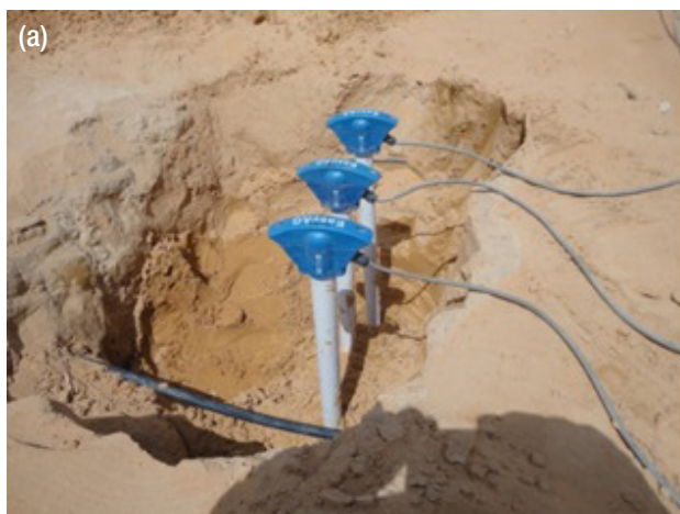
Figure 2. Installation of EasyAG probes in the plot: (a) buried drip line; (b) drip line on the soil surface.
