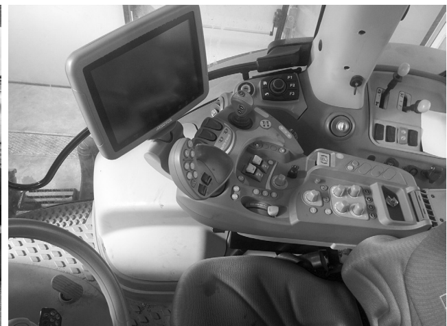
Figure 1. Controls layout in tractors working stations: completely mechanical gearbox with hand lever to select gears and ranges (a), and CVT (b).
