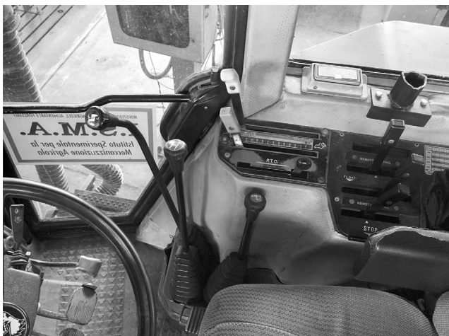
Figure 1. Controls layout in tractors working stations: completely mechanical gearbox with hand lever to select gears and ranges (a), and CVT (b).
