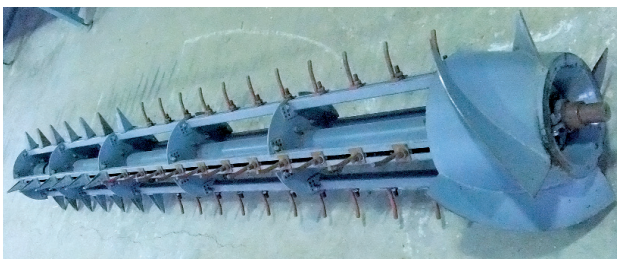
Figure 7. Composite structure of the LFC unit with both spike and trapezoidal teeth.
