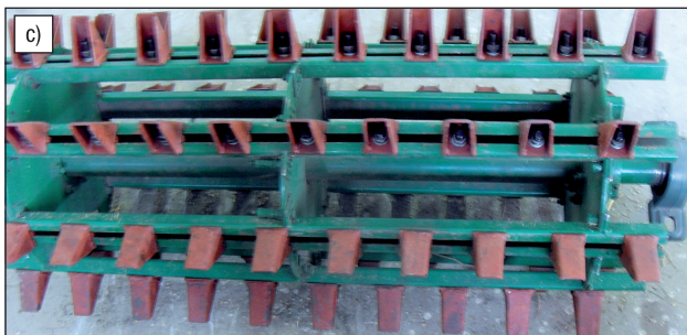
Figure 3. Structural diagram of four threshing tooth TFC unit: (a) spike tooth, (b) knife bar, (c) rectangular bar, and (d) rasp bar.
