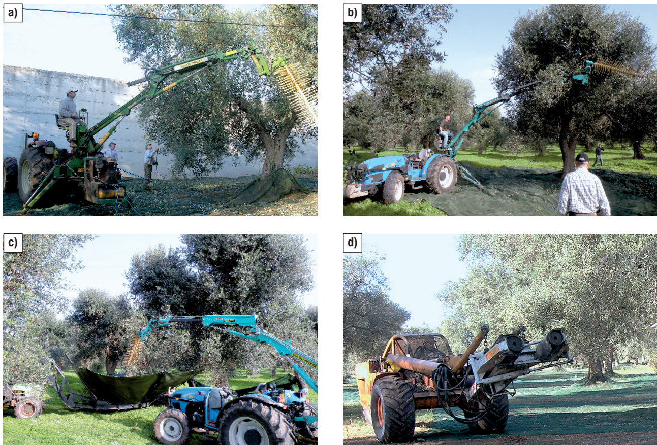
Figure 2. Mechanical beater mounted on a tractor for harvesting: (a) the upper parts of the canopy, plus two hand-held pneumatic combs with handles to harvest the lower parts of the canopy of very large size olive trees used in trial A; (b) the whole canopy plus nets under the tree for collecting the detached olives in Trial C; (c) the whole canopy used in combination with a catching frame (reversed umbrella), mounted on another tractor, for collecting detached olives in Trial C. (d) Self-propelled shaker used in trial B.
