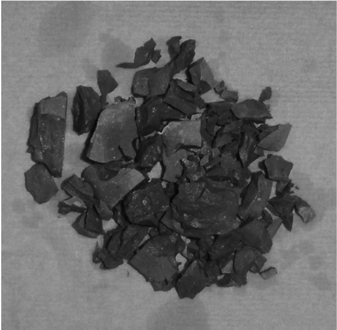
FIG. 3. Picture of the P4-E-3d cement paste after the first 14 cycles.
