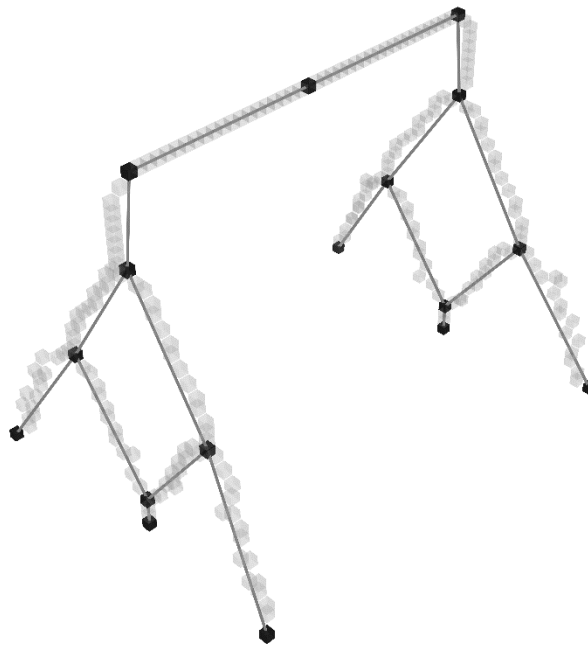
Figure 6: Wireframe (over voxel skeleton in light gray) of the gantry crane model
