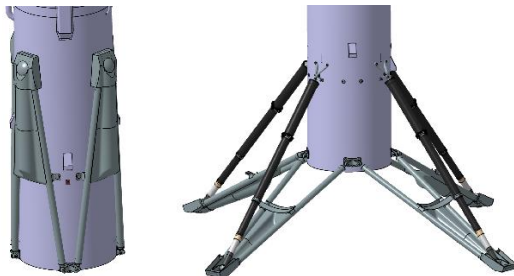
Figure 7: ALS in folded (left) and deployed (right) configuration
