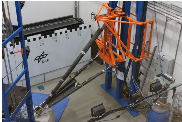
Figure 9: Single Leg Teststand inside LAMA
