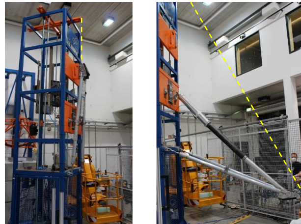
Figure 8: Landing leg at deployment test stand inside LAMA, left: folded, right: deployed
