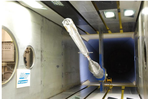
Figure 18: CALLISTO 1:10 scale model with unfolded fins mounted in the HST test setup
