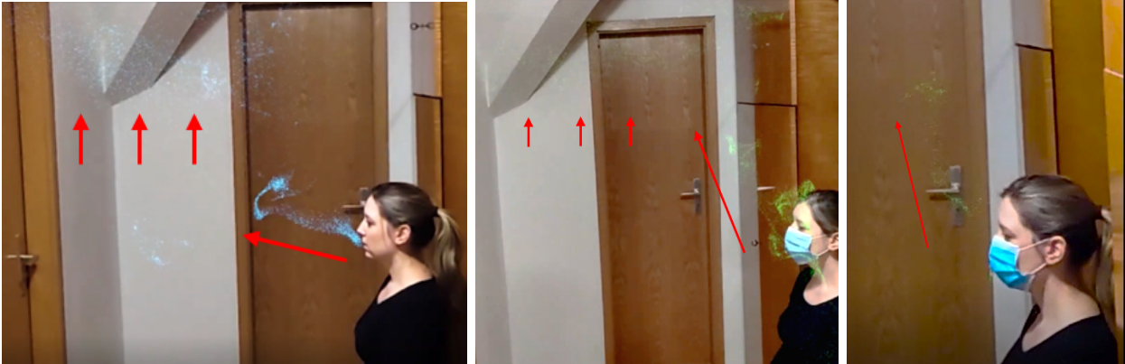
Figure 4: Virtual particle distribution in real environment seen through a HoloLens 2 providing depth perception. Left: In 42 sec, around 40,000 particles are exhaled forwarded without a mask. Middle: Using approx. 80,000 particles in total to better visualize spreading with a surgical mask. Right: Based on tracing results, around 6,500 particles with a surgical mask disperse upwards.
