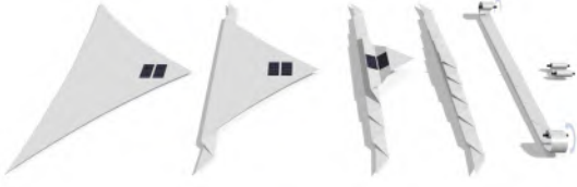
Figure 3: Membrane stowing strategy. As considered in previous concepts, the figure also shows flexible photovoltaic mounted close to the central unit.
