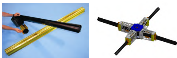
(a) Reelable, tubular double-omega boom in partly deployed state. (b) Breadboard model of the boom deployment unit with four cross-wise aligned booms.
