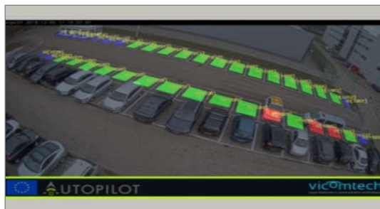
Figure: AVP road unit camera and parking lot detection visualization
