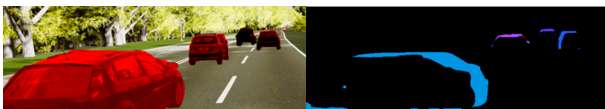
Fig. 5. Disparity vs Entropy. Comparison of the dynamic disparities produced by different objects in motion. Note how observations with high entropy values (brighter red) produce larger shifts of image pixels.
