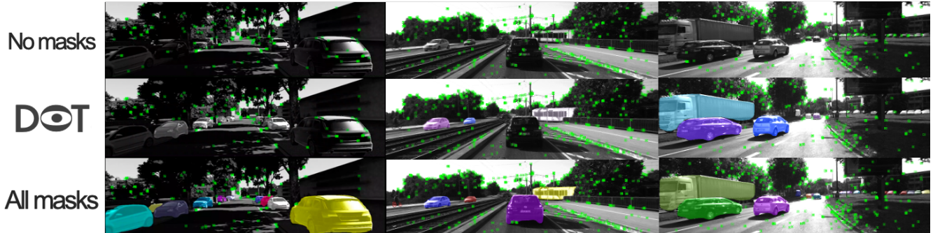
Fig. 1. Top row: ORB-SLAM2 [1] tracks on KITTI [2] images. Middle row: ORB-SLAM2 tracks with DOT segmentation masks, which differentiate between moving and static objects. Bottom row: ORB-SLAM2 tracks using Detectron2 [3] segmentation masks, encoding all potentially dynamic objects. Note how DOT segments out actually moving objects (e.g., moving cars), while keeping the static ones (e.g., parked cars).
