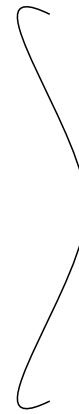
Fig. 2.12: Curved edge treatment to avoid diffractions, taken from [10, p. 988] in side view.
