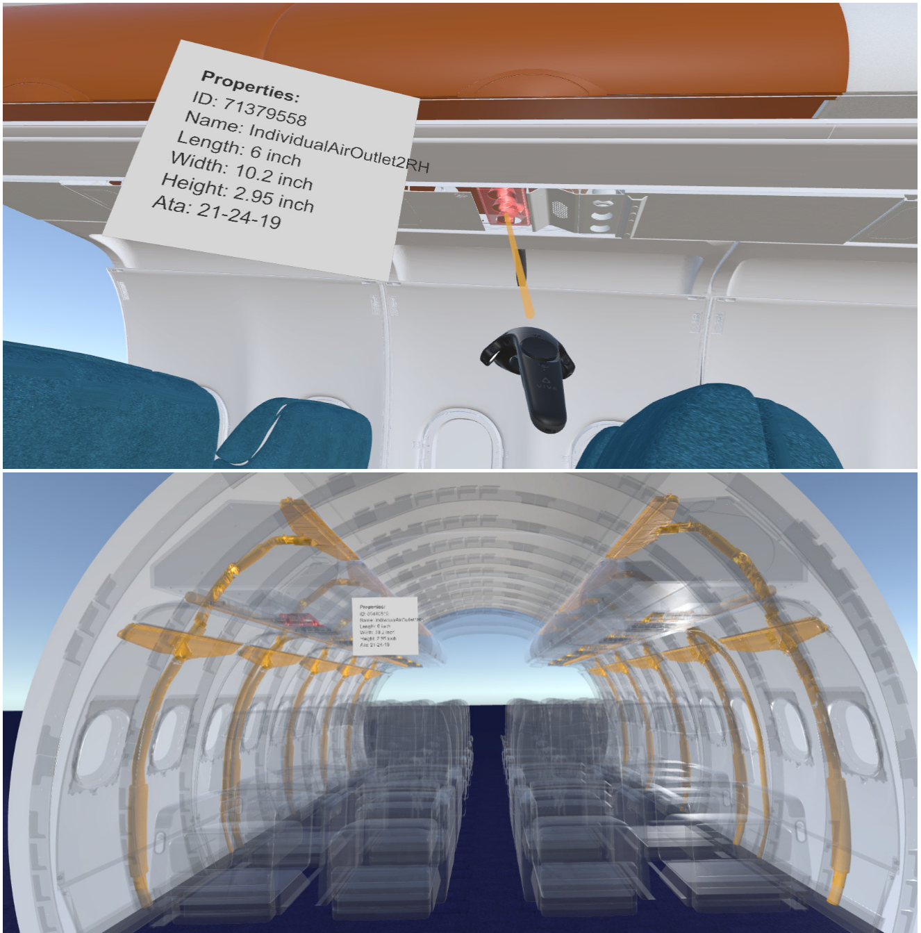
Figure 7 – User view: visualization of the individual air outlet’s properties (upper picture) and the air conditioning system (lower picture).
