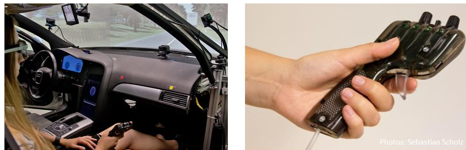
Figure 1. Driving simulator (left) with participant and sensor set-up: MS Band 2 (left), SMI Eye Tracking Glasses 2 (left), and handset control [8] (left and right).
