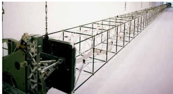
(c) Antennenmast des Space Shuttles Endeavour [68]
