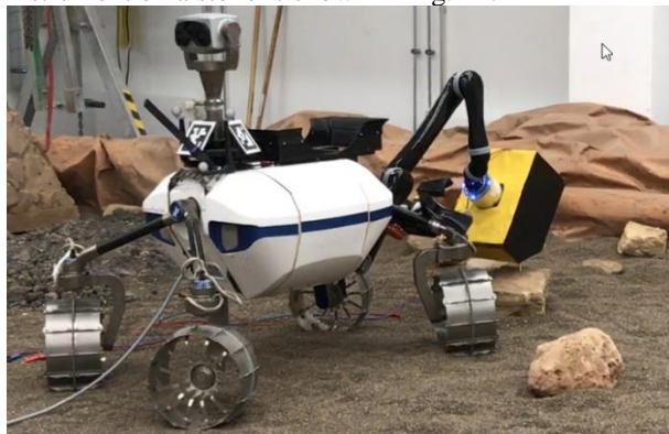
Fig. 12: LRU2 places the LIBS Payload Instrument on stone in the lab
