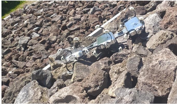
Fig. 25: The Scout rover making its way up a 30 degrees sloped boulder field
