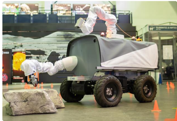
Fig. 22: INTERACT rover with covers and sleeves for dust protection
