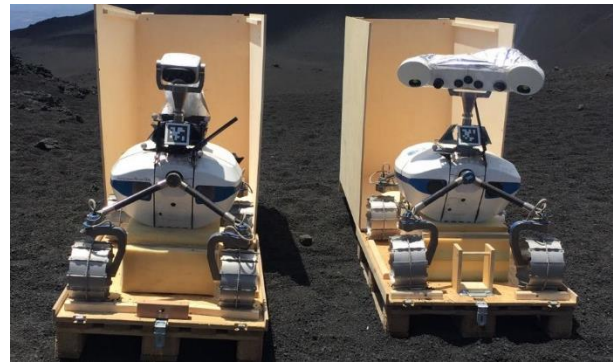
Fig. 27: LRU 2 equipped with cameras mainly used for navigation and manipulation, right: LRU 1 equipped with additional cameras supporting scientific analyses
