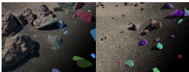
Fig. 14: Example images of synthetic training data generated by OAISYS
