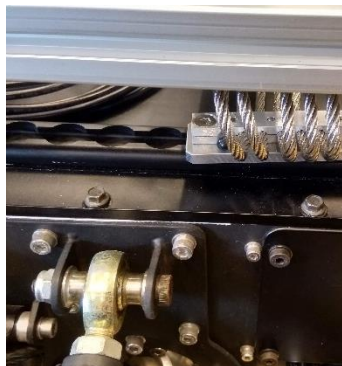
Fig. 24: A wire spring damper to decouple the stiff payload container from the locomotion unit
