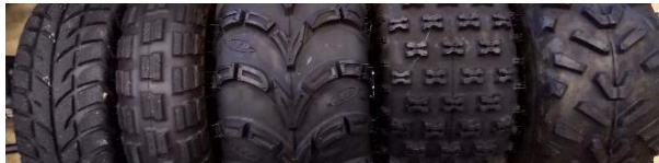
Fig. 23: Tire options for Mt. Etna (left: road tire, mid: contenders, right: the choice for Mt. Etna)
