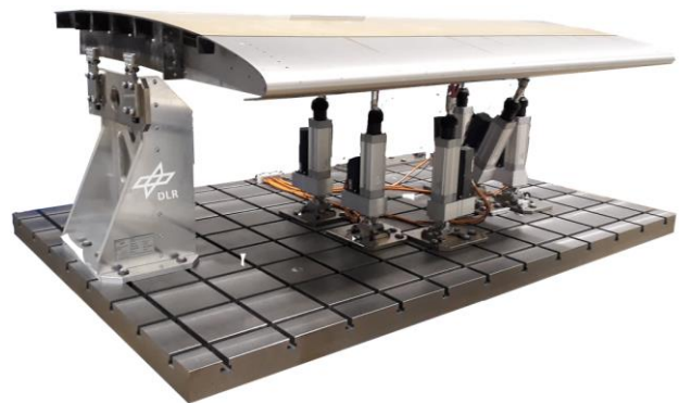
FIGURE 7. Full GBD with leading edge, integrated in the test stand (partial view).
