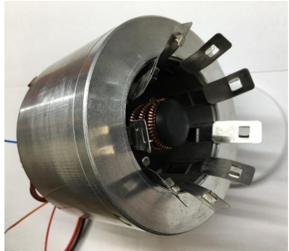
Fig. 3. Active Coupling Partner with spring elements opened-up.
