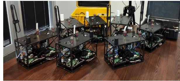
Fig. 21. Seven RC-LOFAR modules assembled and integrated to the PBIMS in each module.
