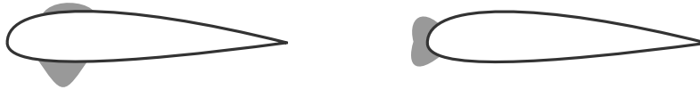
Figure 4: Schematic illustration of the App. C wing ice shape configurations: run-back ice (left) and leading-edge ice (right).
