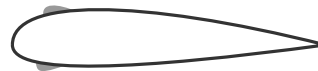
Figure 5: Schematic illustration of the artificial wing SLD-ice shapes (not to scale) used for all three SLD configurations.
