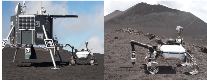
Fig. 1 Two operation scenarios of the LRU during the 2017 Etna Moon Analogue Campaign [10]: Collection of scientific equipment from a lander (left) and deployment of a geophone in the ground (right). Credit: DLR.
