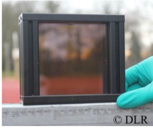
Fig. 6. Image of switchable photovoltaic window with 25 nm \text{MgH}_2 in transparent state.
