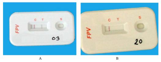
Fig A. Result window of test kit showing two colour bands (C and T) indicating Feline Panleukopenia Virus (FPV) positive result (sample no. 03) and Fig B. showing only one colour band (C) indicating Feline Panleukopenia Virus (FPV) negative result (sample no. 20).
