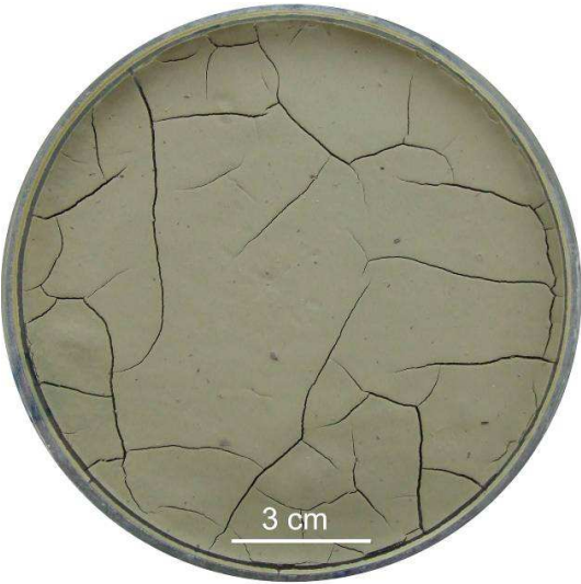
28 29 Fig. 2 A typical desiccation crack pattern of specimen during the first 30 drying path
