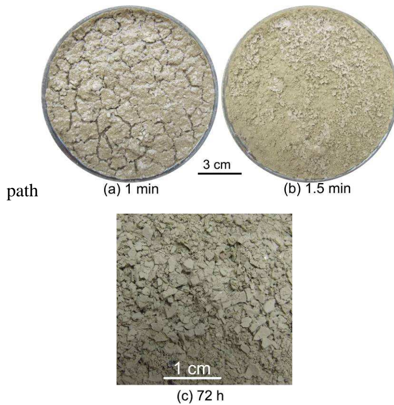
Fig. 10 Evolution of surface cracks during the third wetting path
