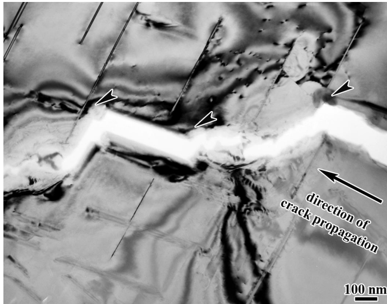
Fig. 4.13. Path of a crack propagating through a field of Al 2 Cu plates. The arrow indicates the original crack opening direction, which was deflected as separation occurred in the matrix region in between plates.
