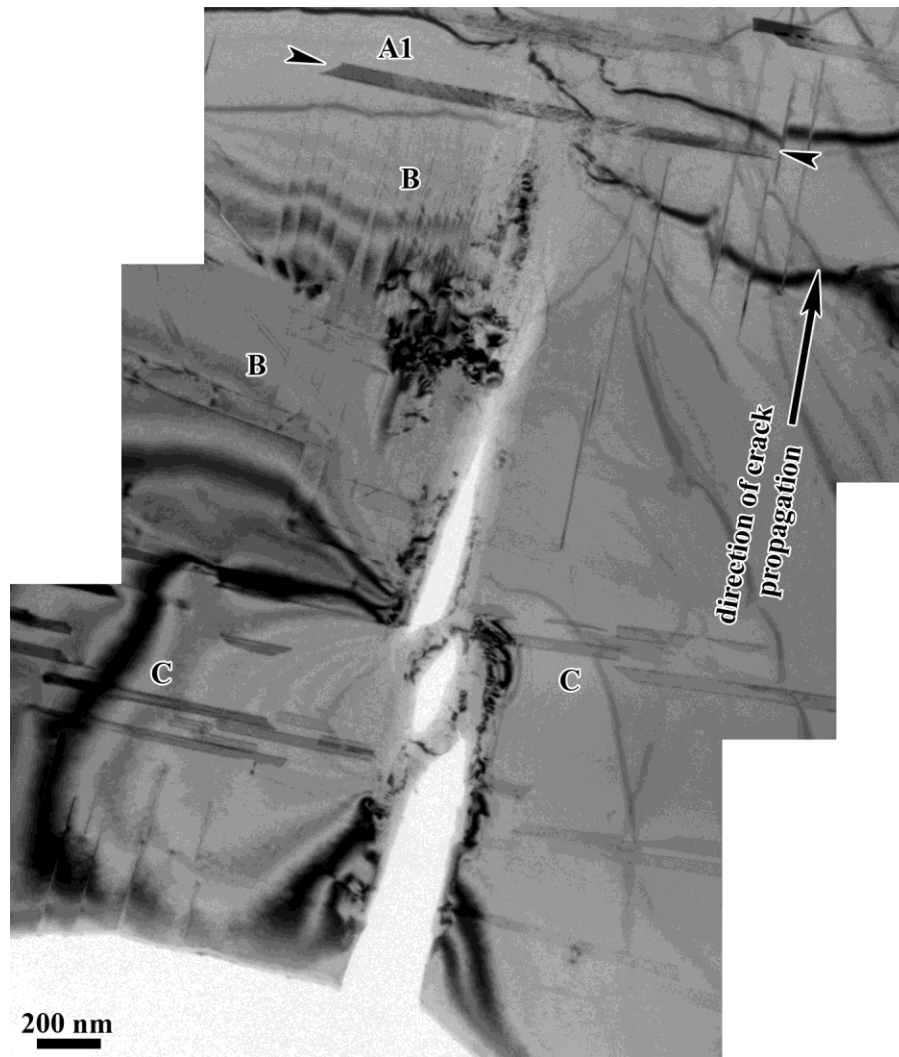
Fig. 4.2. The dislocation-emitting crack from Fig. 4.1 after in situ straining. The first sheared Al 2 Cu platelet 'A1' is denoted by arrowheads. Regions labeled 'B' show a predominance of the same slip traces left by dislocations seen in Fig. 4.1. Smaller particles of the same orientation as 'A1' are present in the thinner regions of the foil, labeled 'C,' which did not interact with the crack.
