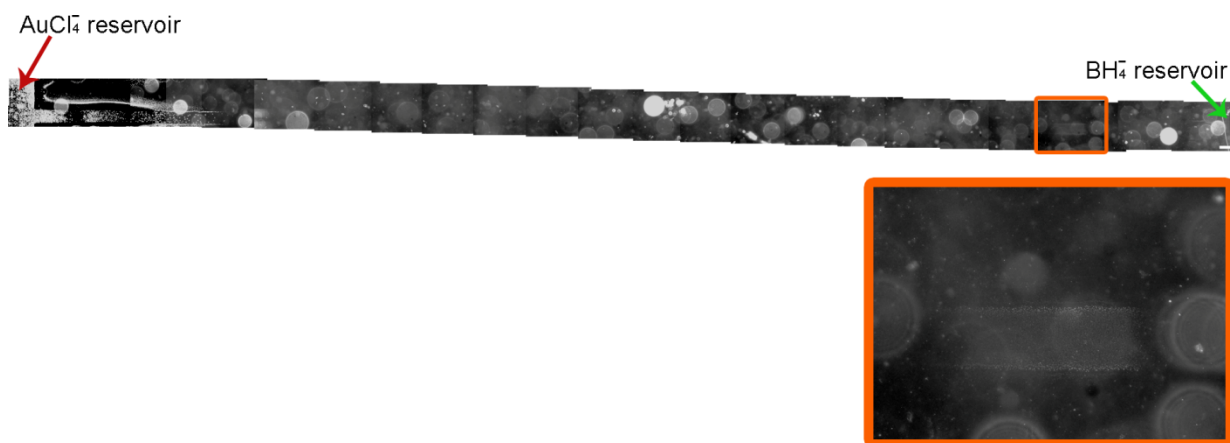
Figure 3. 6. Dark field optical image of \text{AuCl}_4^- and \text{BH}_4^- transportation along the linear POEGA pattern and Au nanoparticles formation in a dilute system (aqueous solutions were prepared in pH 6 buffer). Scale bar is 100 \mu\text{m} .
