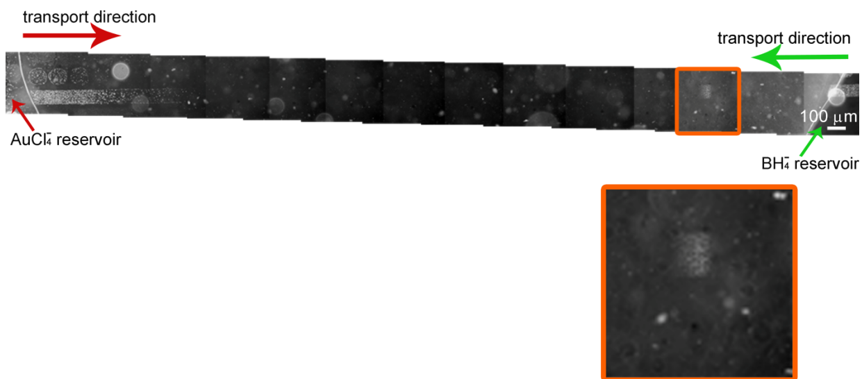
Figure 3. 5. Dark field optical image of \text{AuCl}_4^- and \text{BH}_4^- transportation along the linear POEGA pattern and Au nanoparticles formation (aqueous solutions were prepared in pH 2 buffer).
