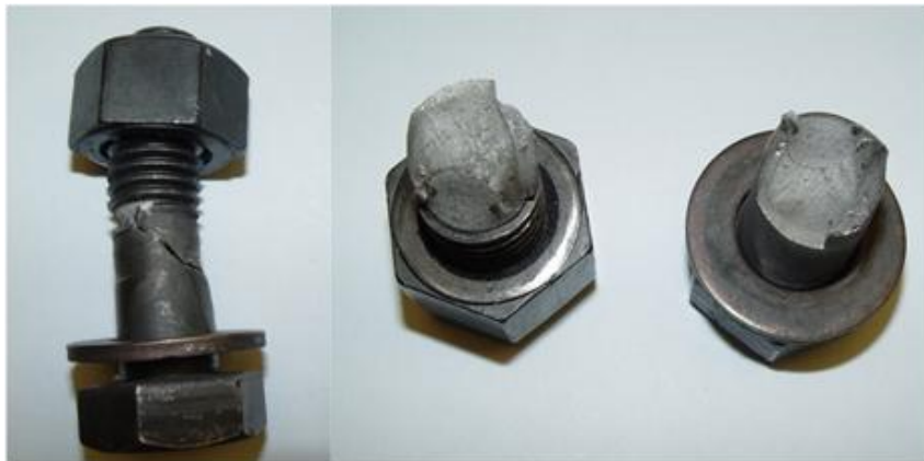
Figure 4-41 Shear failure of bolt 2 including failure surface characterized by shear lips during cyclic testing of the 50% M_{p_{beam}} connection
