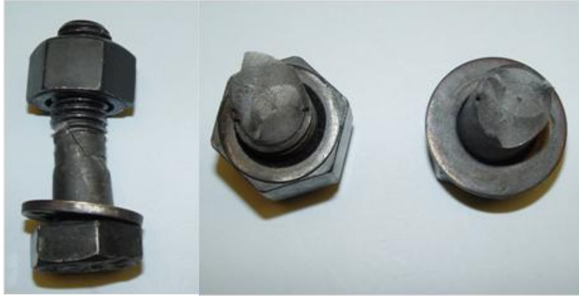
Figure 4-42 Shear failure of bolt 4 including failure surface characterized by shear lips during cyclic testing of the 50% M_{p_{beam}} connection
