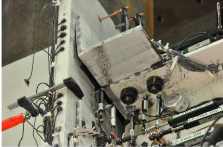
Figure 4-46 Deformation of the specimen during the post-earthquake cyclic testing of the 30% M_{p_{beam}} connection
