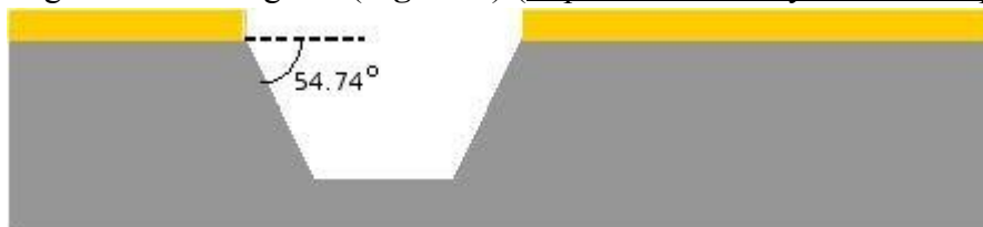
Figure 5. Diagram of anisotropic etching of a Si[100] surface. The yellow layer represents a mask patterned over the gray layer of Silicon. Once the etchant begins etching the Si layer, it etches down at an angle of 54.74 degrees. Other anisotropic etching angles are achievable with surfaces of different atomic structure and/or orientation ( http://cleanroom.byu.edu/KOH.phtml ).
