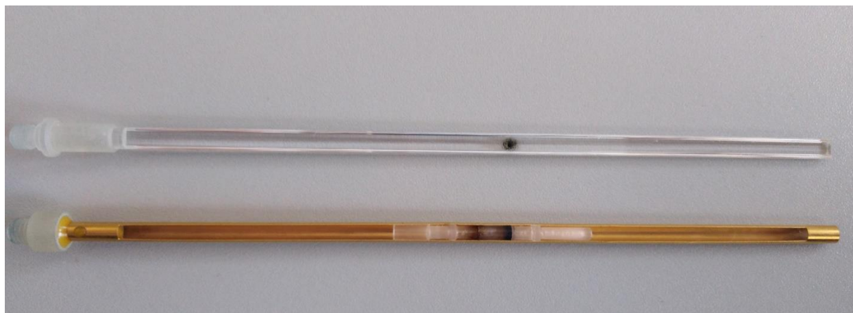
Figure 2.7.1 Quartz (up) and brass (down) holders with drop-casted sample and sample in capsule resp.
