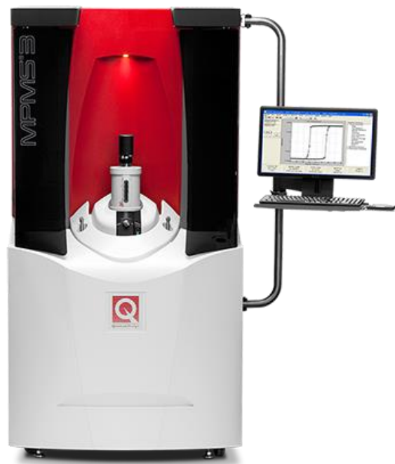
Figure 2.5.1 MPMS 3 SQUID commercially available by Quantum Design. This type of magnetometer was used in the majority of the magnetic measurements conducted in the framework of this thesis, thanks to the permission of Dr. Anja Wolter-Giraud. The image is reproduced from www.qdusa.com
